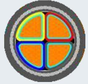
**Four core Fire resistant cable, Copper conductor, Glass mica taped, XLPE insulated, Gal. steel wire armoured, LSF/LSZH sheathed, 600/1000V, conf. to BS: 7846**
