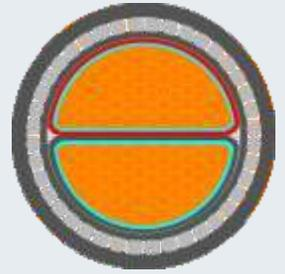
**Two core Fire resistant cable, Copper conductor, Glass mica taped, XLPE insulated, Gal. steel wire armoured, LSF/LSZH sheathed, 600/1000V, conf. to BS: 7846**
