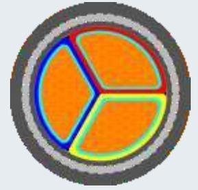
**Three core Fire resistant cable, Copper conductor, Glass mica taped, XLPE insulated, Gal. steel wire armoured, LSF/LSZH sheathed, 600/1000V, conf. to BS: 7846**
